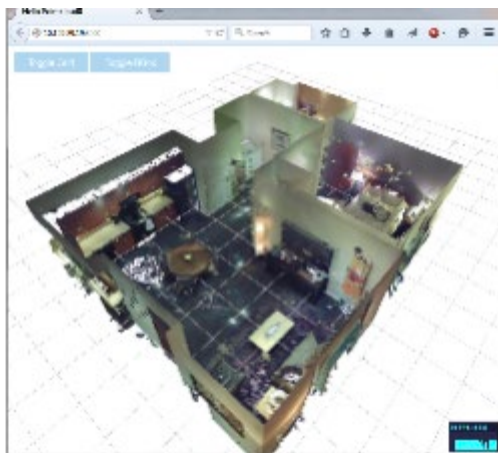
Fig 1: Prototype of the web-based viewer, running inside the Chrome browser and displaying the point cloud created from SON's simulated apartment.
